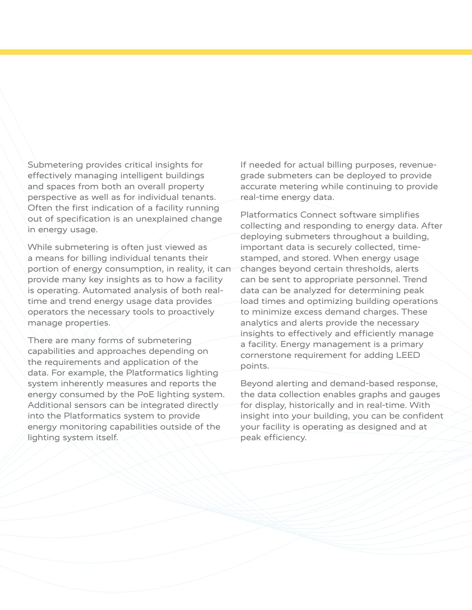
Submetering provides critical insights for effectively managing intelligent buildings and spaces from both an overall property perspective as well as for individual tenants. Often the first indication of a facility running out of specification is an unexplained change in energy usage.
