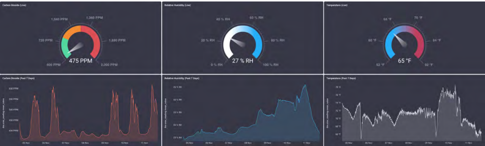
Dashboard featuring live gauges of current sensor levels and trendline graphs of the past 7 days.
